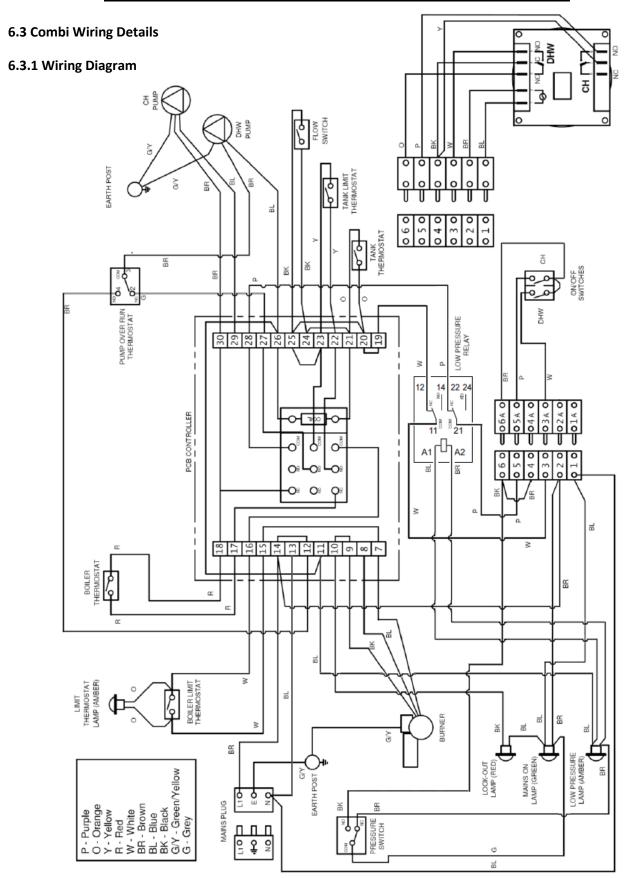
The 3 pin mains plug must be supplied with a permanent live to allow the pump overrun stat and relay to operate.
