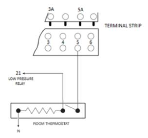
Remove the purple wire from terminal 5 on the terminal strip, and terminal 21 on the low pressure relay, then connect the thermostat as shown.
